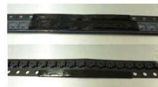
Embossed tape complete example
