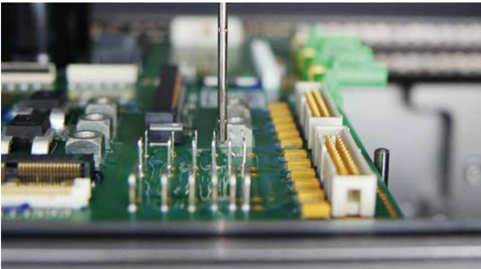
Precise coating of electronic connections between tightly packed, tall components
