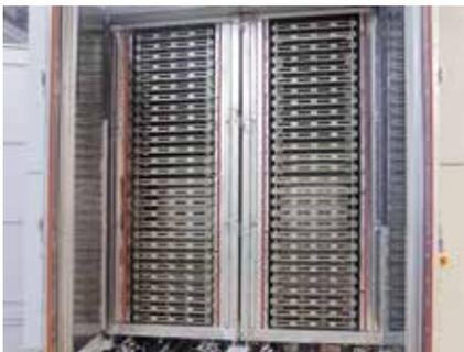
Vertical stacking principle in the process towers for receiving the goods carriers
